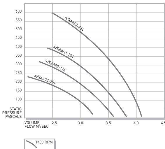
▼ **Type A/SAA fans** are designed for use in ducted exhaust applications. Each impeller is individually designed and manufactured to precise specifications for maximum airflow at high pressure levels.
